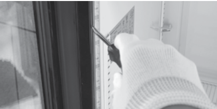
1 Use a screwdriver to pry the light bar out of the slot.
