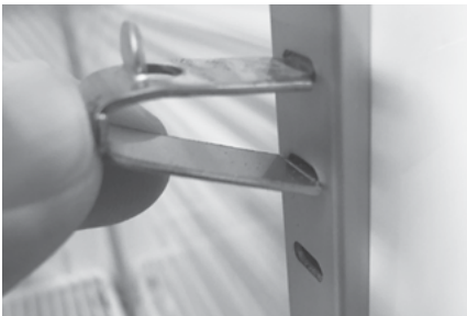
Securely insert shelf clips into pilasters
