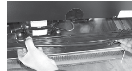
2. The back metal grill can now be removed.
