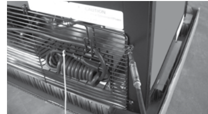
1. Using a Phillips screwdriver, remove the (4) screws from the back grill as shown.
