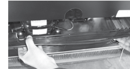
2. The back metal grill can now be removed.
