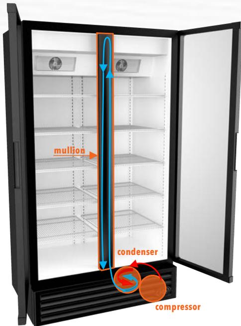
A simplified overview of the refrigerant flow in a Cooler with a mullion is as follows:
