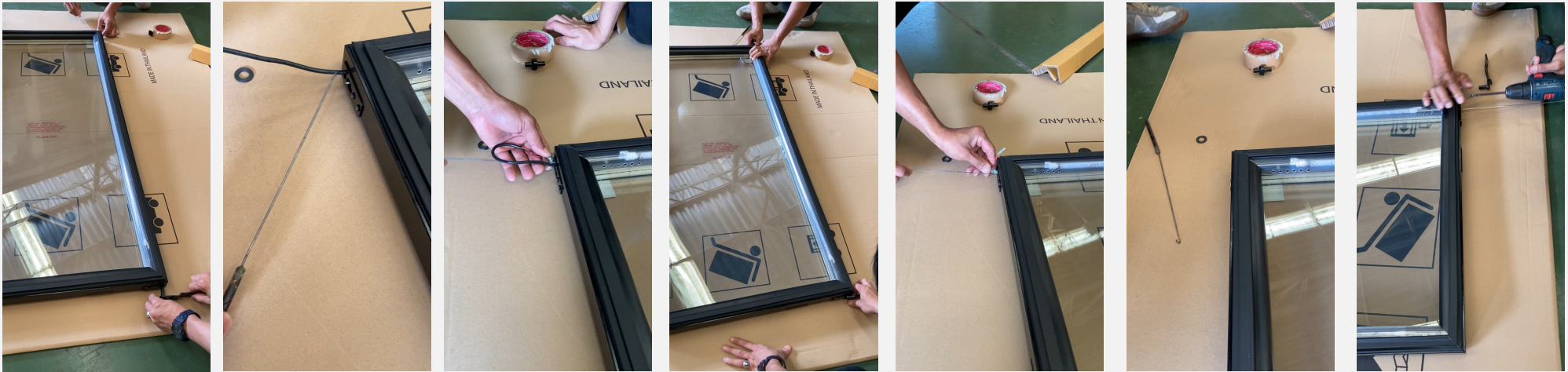
Attaching the wire connector to the wire tension spring (videos).
