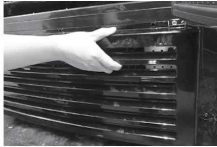
2 The front grill can now be removed by pulling it out.
