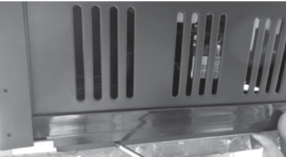
1. Using a Phillips screwdriver, unscrew the (2) screws at the base of grill.
