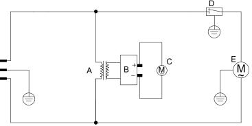
A. Control board B. Storage battery C. Evaporator fan
